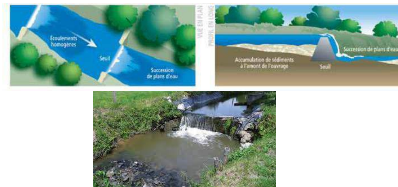
Figure 5-11. Typical weir's structure.
