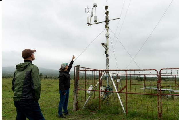
An Eddy Covariance, which is part of the research infrastructure at ILRI's Kapiti Research Station and conservancy is being used to measure ecosystem carbon exchange to determine whether the savanna ecosystem is a source or sink of carbon
