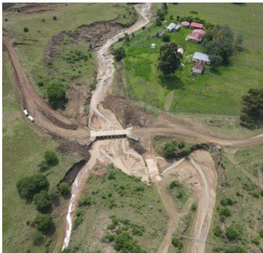
Figure 4-5: Example of erosion and flood extent threatening a bridge in Alfred Nzo DM
