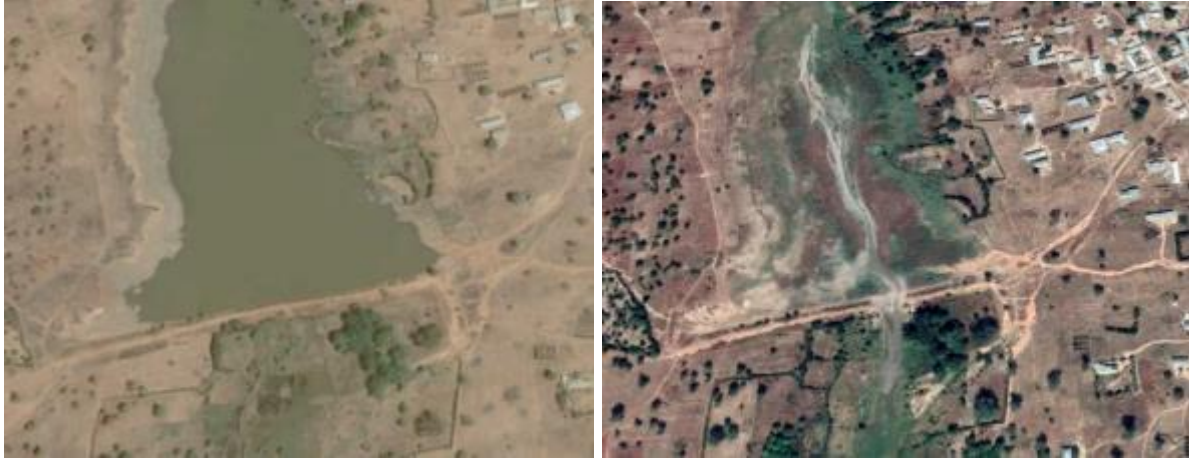
Figure 60. Example of a dam breach in the Upper West region, west of Nawdoli. Left: February 2020, Right: November 2021. Obtained from Google Earth.
