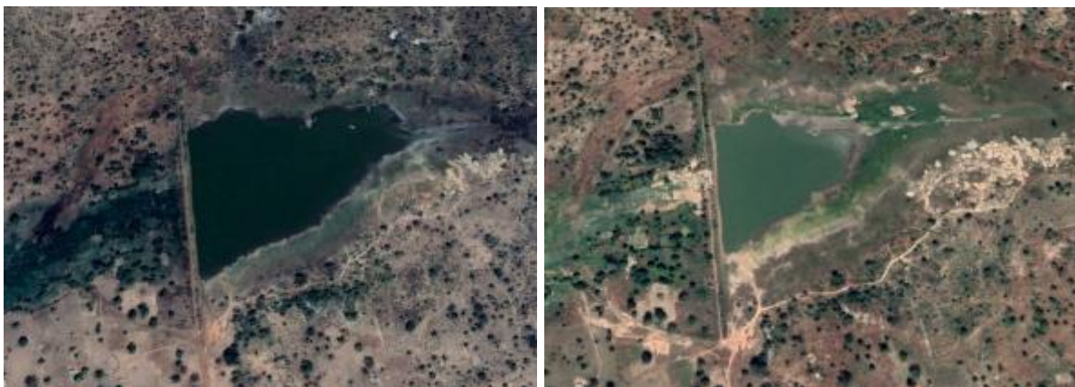
Figure 61. Example of a dam breach in the Upper West region, north of Moyiri. Left: April 2021, Right: November 2021. Obtained from Google Earth.
