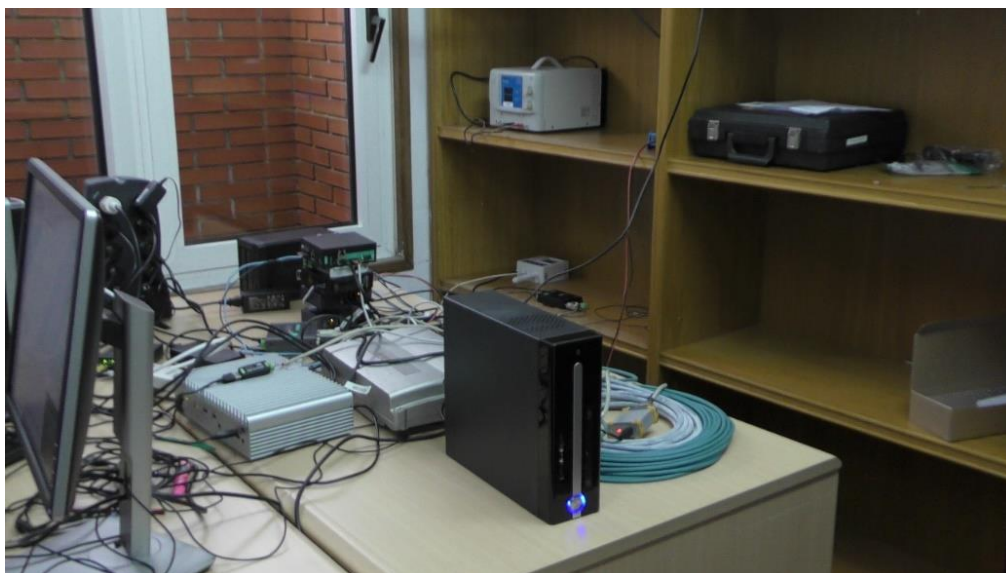
Figure 19. Land installation including an engine simulator to test devices and to perform preliminary configuration within SusTunTech project.
