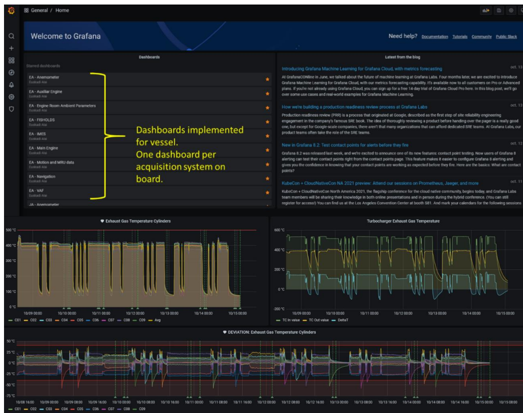
Figure 20. Dashboards configured for the easy monitoring of data flows in real-time used in SusTunTech project.
