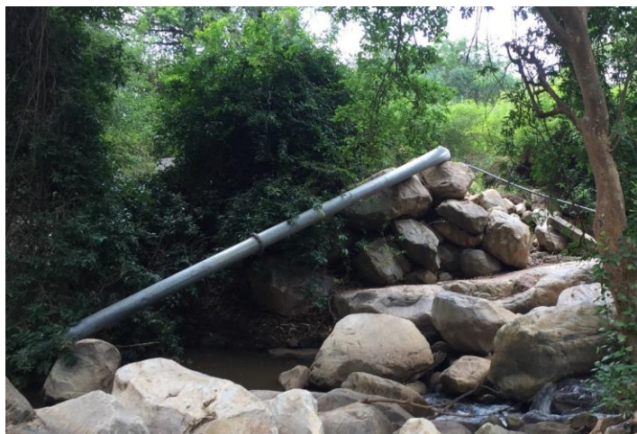
Plate 13.9: Destroyed Section of GI Pipeline
