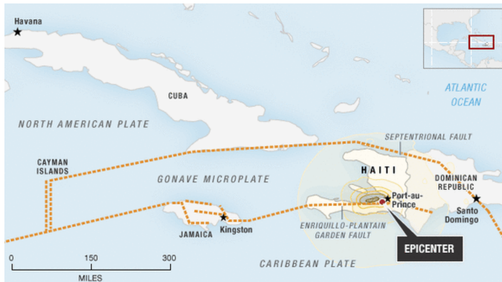
Figure 2. Image illustrating the Septentrional and Enriquillo-Plantain Garden Faults which run through Haiti, as well as the epicentre of the earthquake which occurred in 2010 54 .
