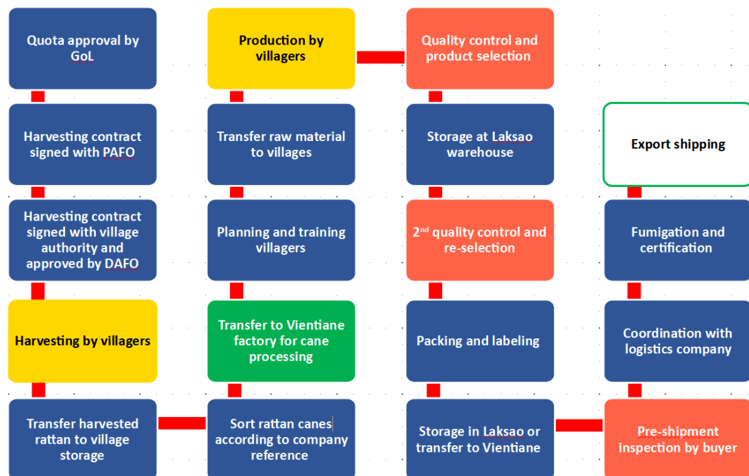
Figure 23: Project production process for rattan baskets. (Based on Thammavong and Vongkhamsao, 2018)
