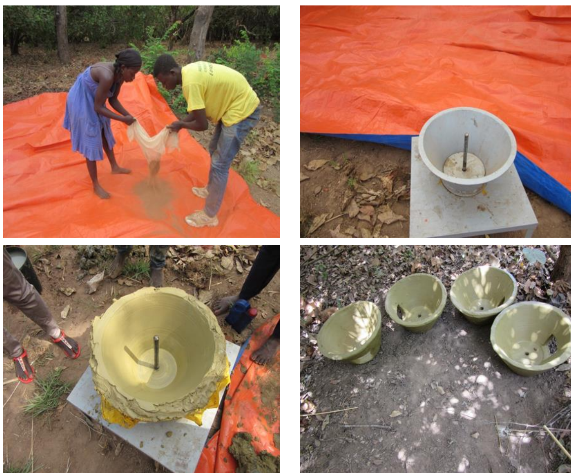
Picture 14. Clay part of the stove production process. The metal part is produced by artisan blacksmiths who reuse existing metal sheets/plates.
