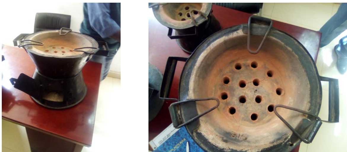
Picture 13. Charcoal saving cooking stove – model approved and recommended by INITA
