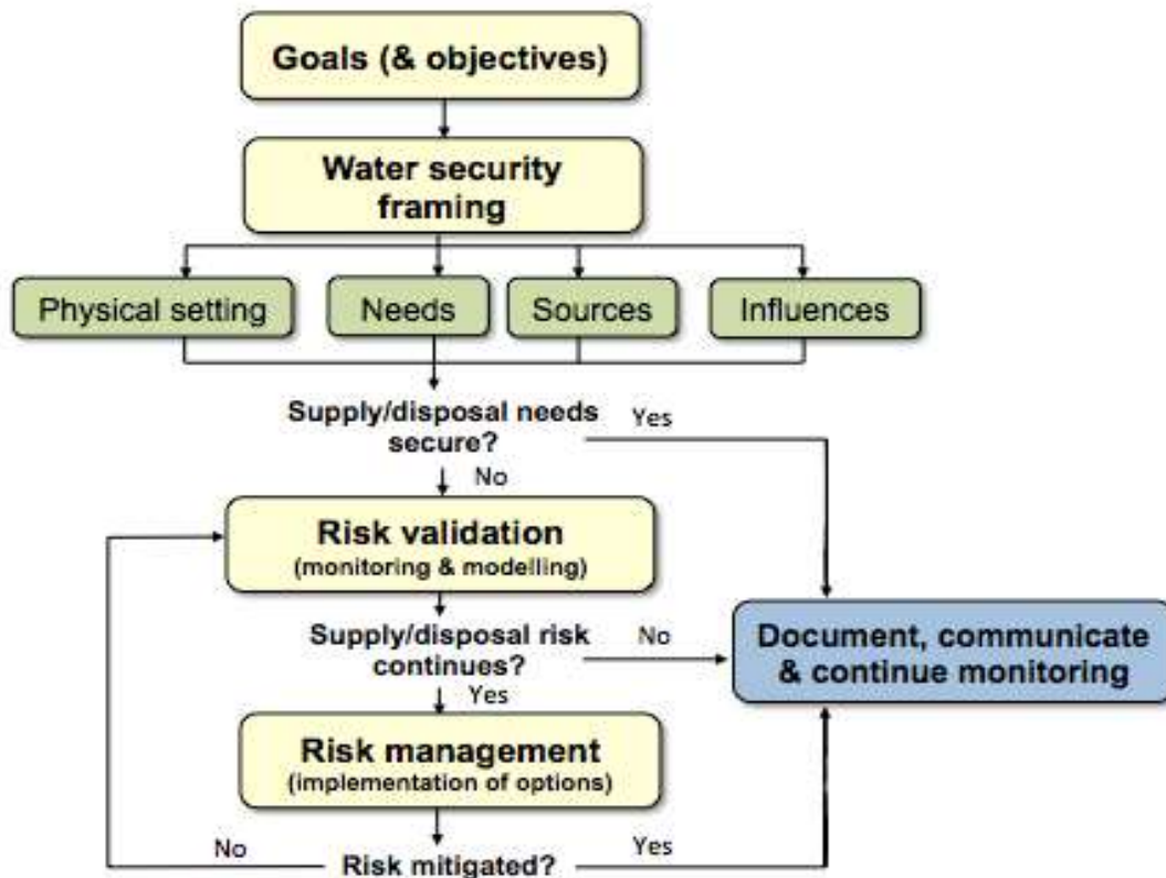
Figure W. Process Flow for Water Security Assessment
