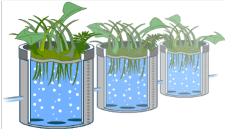
Figure K. Illustration of Plants Growing above Bacterial Bioreactor Tanks in a Solar Aquatics System
