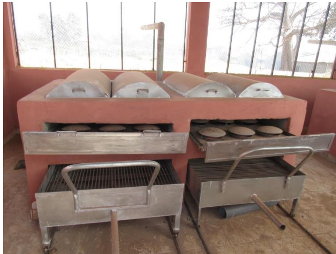
Figure 16 –FTT ovens of artisanal construction – Very poor materials and standard of fabrication
