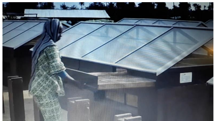
Figure 8 The CEAS Kiraye solar drier in use throughout Senegal
