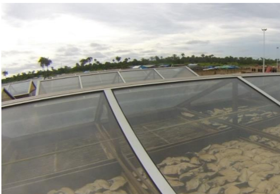
Figure 8 The CEAS Kiraye solar drier in use throughout Senegal
