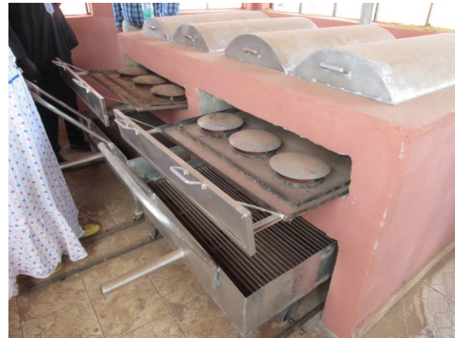
Figure 16 –FTT ovens of artisanal construction – Very poor materials and standard of fabrication
