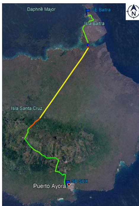
Figure 37. Layout of 34.5 kV sub-transmission line
