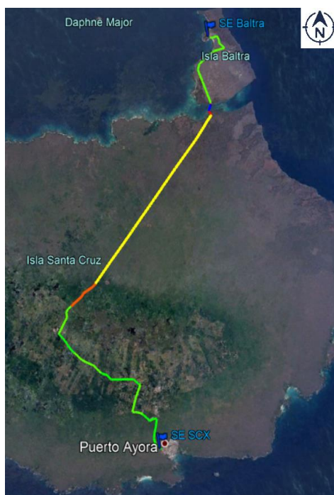
Figure 37. Layout of 34.5 kV sub-transmission line
