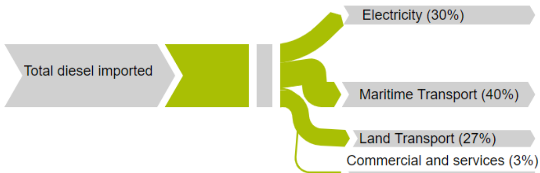
Figure 1. Sankey Diagram of total diesel consumption by sector.
