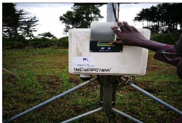
Figure 62: Automatic Weather Station, Sasumua Dam: (Data logger not functional due to lack of battery)
