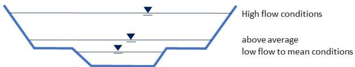
Figure 12: Standard cross-section with berms
