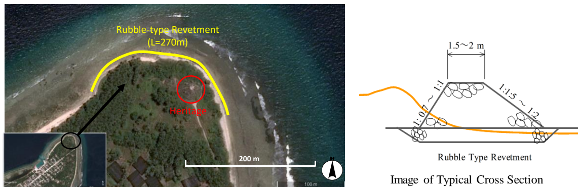
Figure 8.3.8 Coastal Protection Measure at Ishdhoo Island in Laamu Atoll
