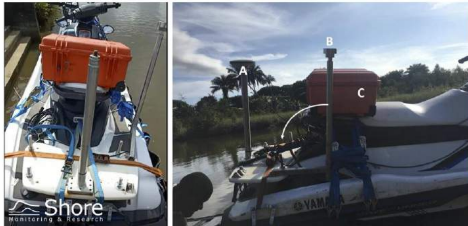
Figure 2.4: Instrument setup modular SBES system on local jetski. RTK-GNSS antenna (annotation A), SBES (annotation B) and survey kit (annotation C).
