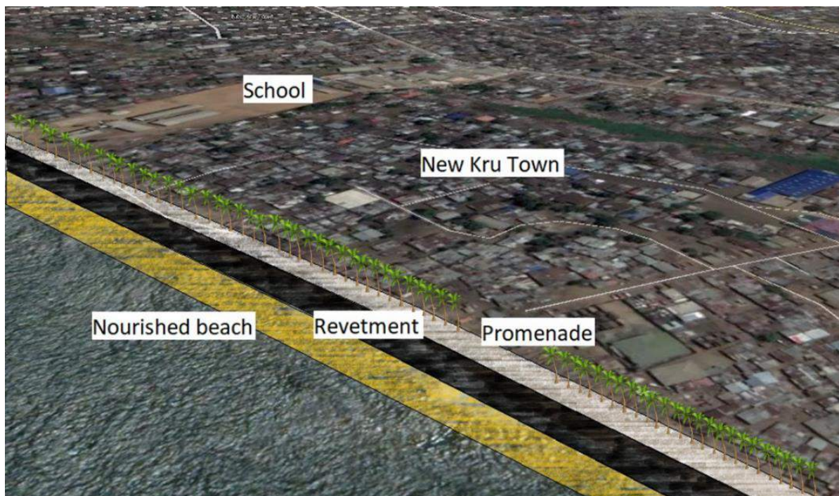
Figure 7-5: Revetment with a nourished beach
