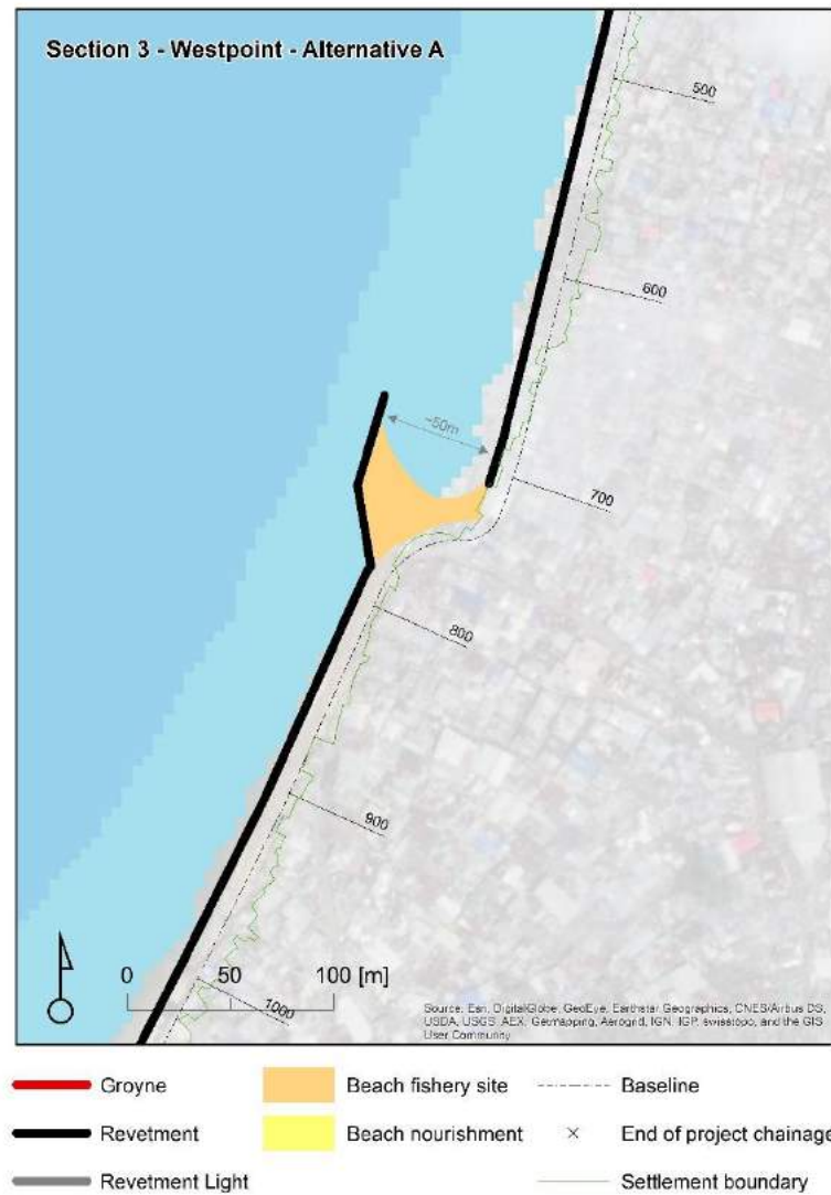
Figure 3-16: Principle of fishing landing site middle part West Point (Chainage 700m)
