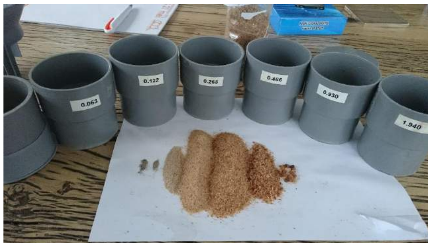
Figure 8-6: Sieving to assess particle size distribution
