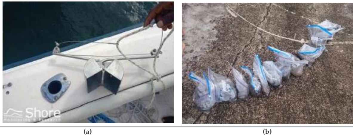
Figure 5-19 (a) Van Veen grab sampler; (b) Sediment samples collected in plastic bags
