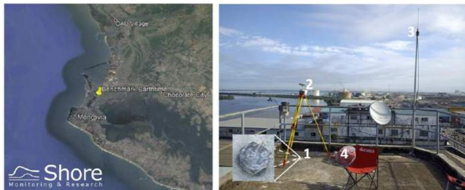
Figure 2.1: Creation of new benchmark. Left panel: Location of benchmark. Right panel: survey bolt drilled into concrete (annotation 1). Tripod with RTK-GNSS positioned above the bolt (annotation 2). Extended radio antenna to increase the area where RTK-GNSS corrections can be received (annotation 3). Leica RTK-GNSS; logging raw observations during creation of benchmark, later on used as base station (annotation 4).
