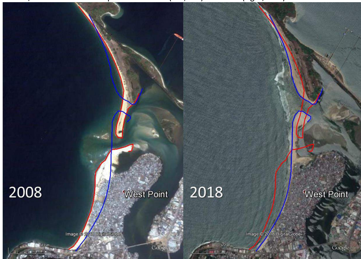
Figure 0-1: Observed coastal retreat at West Point, showing the coastline in 2008 (red) and 2018 (blue)
