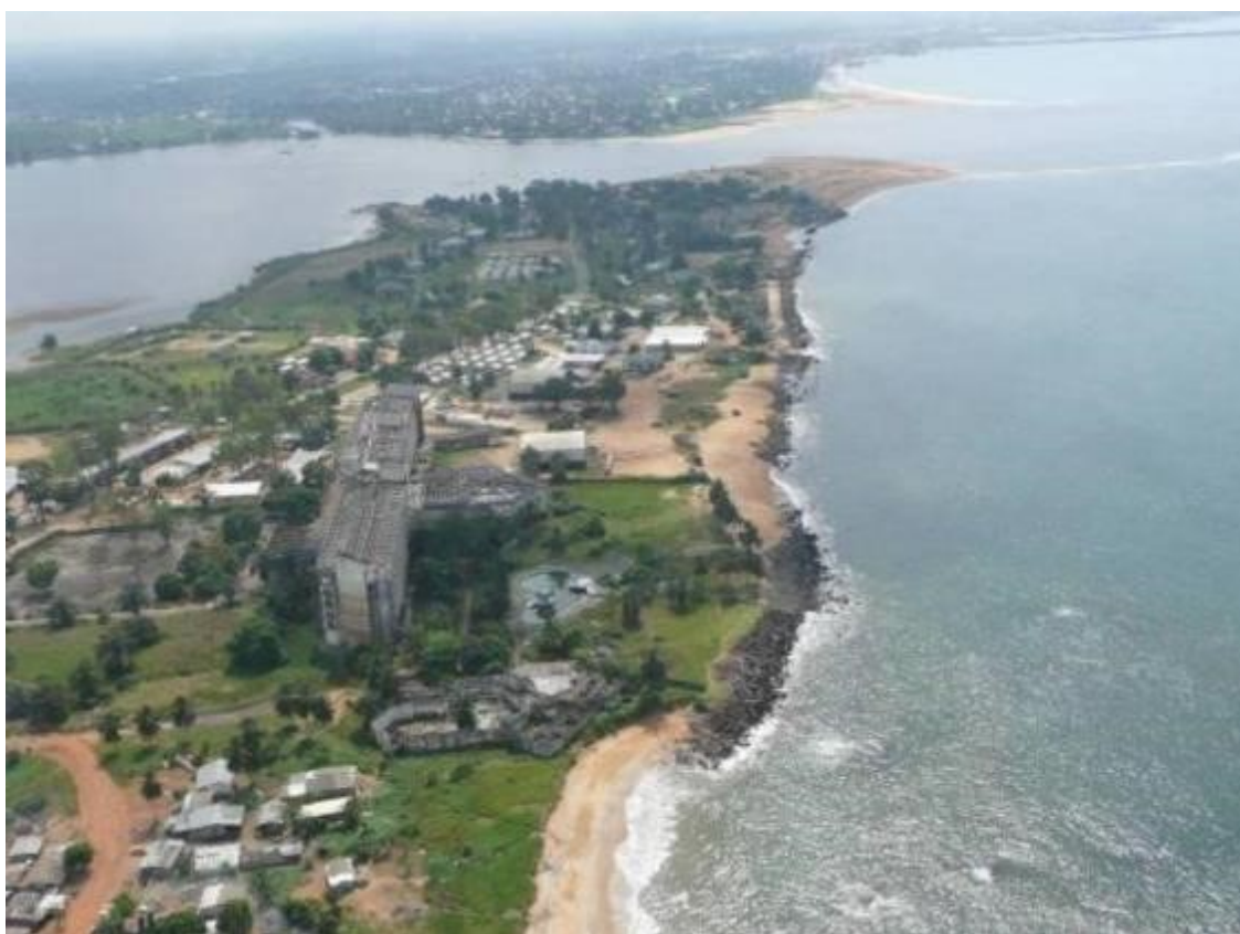
Figure 48. Aerial photo of Hotel Africa area with mouth of St. Paul River at the far stretch. The existing rock revetments established with private funding are visible in the foreground of the photograph.
