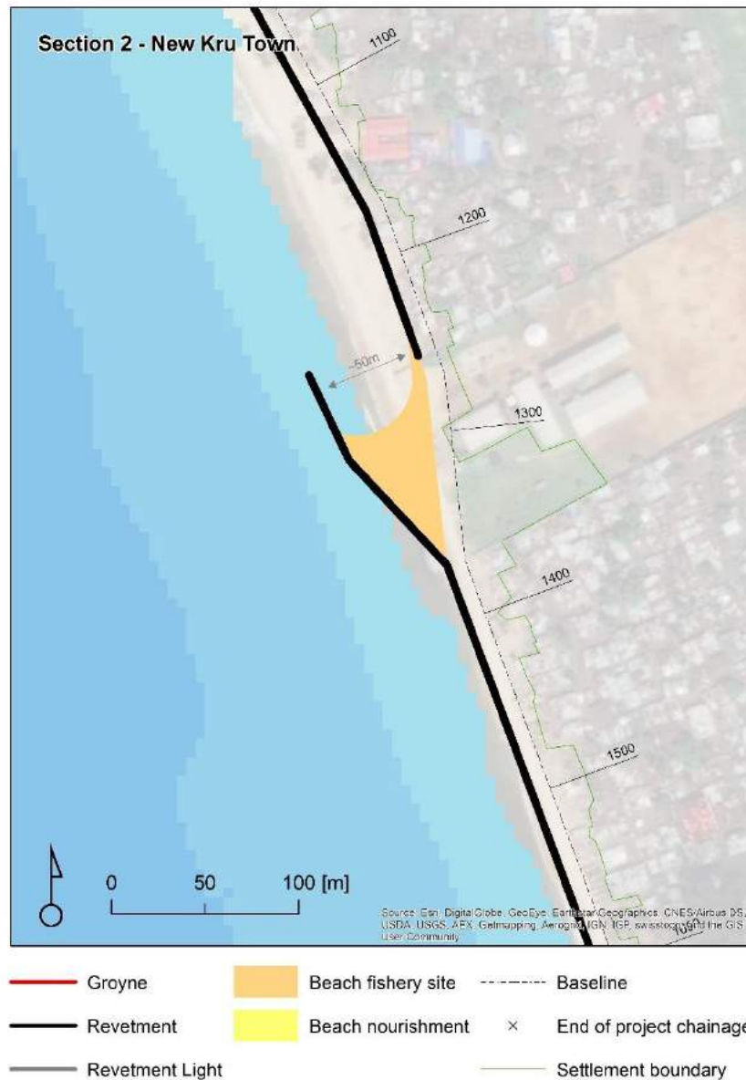
Figure 3-7: Principle of fishing landing site northern part New Kru Town (Chainage 1350)
