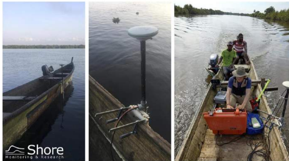
Figure 2.5: Instrument setup modular SBES system on local boat.
