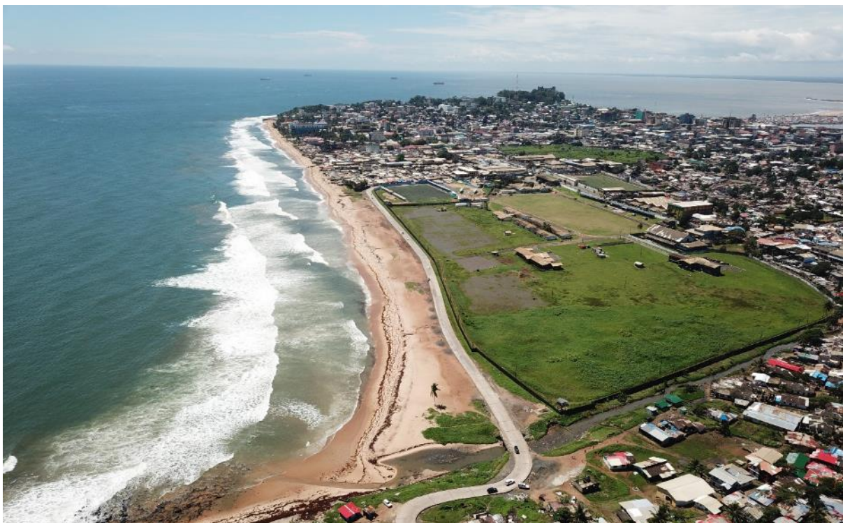
Figure 5-33 Main sewage outlet of Monrovia (down centre of the photo) discharging raw wastewater to the south of the Barclay Training Center beach (coastal section 4)
