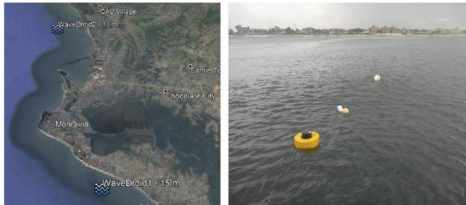
Figure 2.7: WaveDroid deployment. Left panel: Indication of WaveDroids. WaveDroid1 in front of the JFK Hospital beach and WaveDroid2 in the vicinity of the Hotel Africa and New Kru Town beaches. Right panel: Deployed WaveDroid1.
