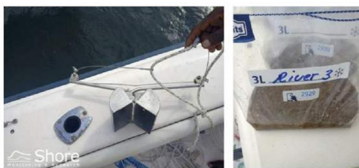
Figure 2.9: Sediment samples. Left panel: Van Veen Grabber. Right panel: sediment sample secured in plastic zip-lock bag.
