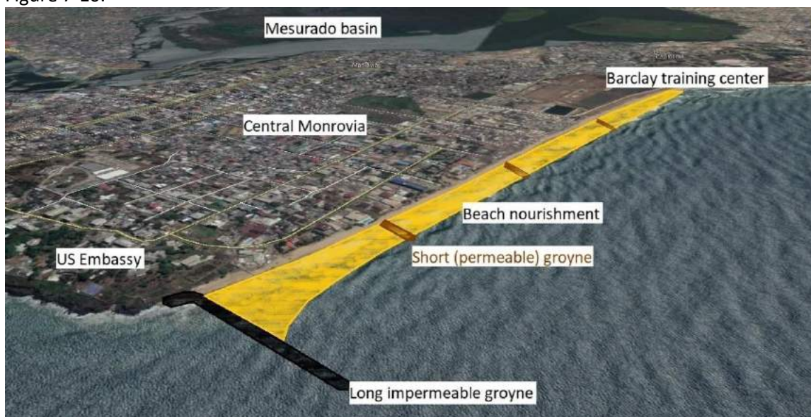
Figure 7-10: Long groyne with a wide sustainable beach including short (permeable) groynes
