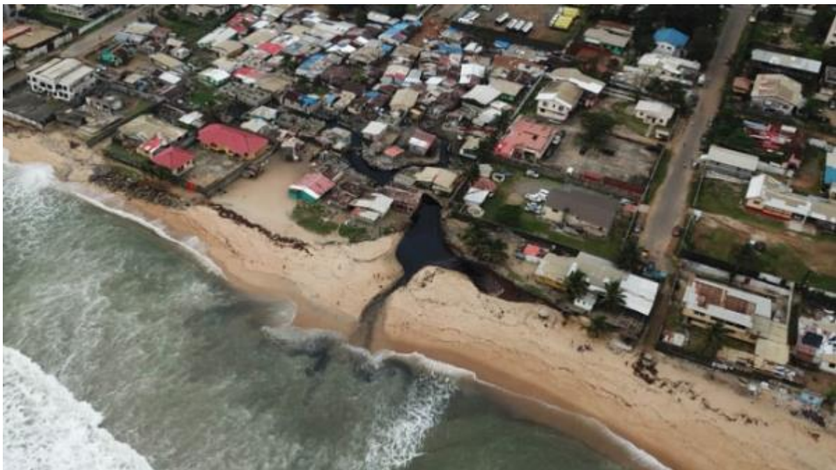
Figure 5-13 Sewer outlet in coastal section 5 discharging raw wastewater in the Atlantic Ocean
