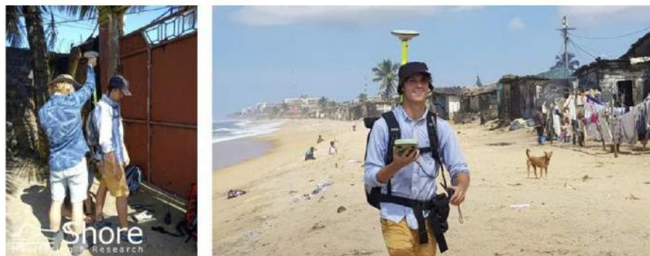
Figure 2.6: Topographic survey. Left panel: measuring vertical offset between GPS antenna reference point and ground. Right panel: surveyor walking on the beach.
