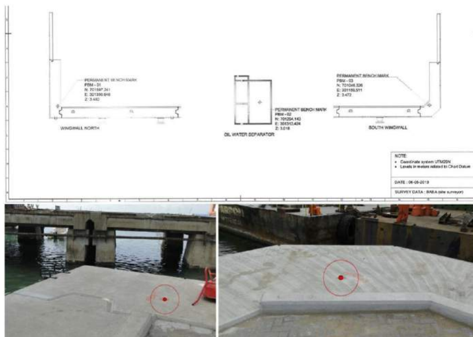
Figure 3.1: Overview of BAM benchmarks in coping beam of quay (top). Benchmark PBM-01 (left) and PBM-03 (right)
