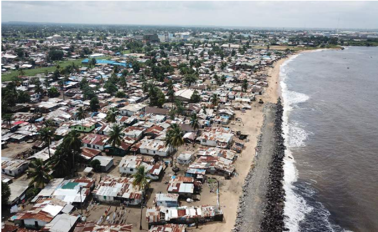
Figure 1-5: Stone pitching of the foreshore at New Kru Town in 2018. Although stated as a revetment, resource constraints are such that this structure lacks the characteristics of a genuine revetment as normally defined in civil engineering. Nevertheless, it is adequate to protect the settlement for at least some years under present sea conditions.
