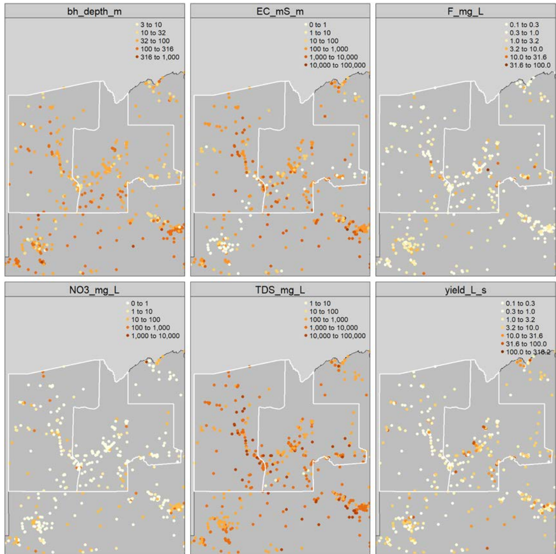
Figure 33. Borehole water depth, yield, and quality (electrical conductivity, F, NO 3 total dissolved solids) in Ngamiland. Data source: Botswana Department of Water Affairs
