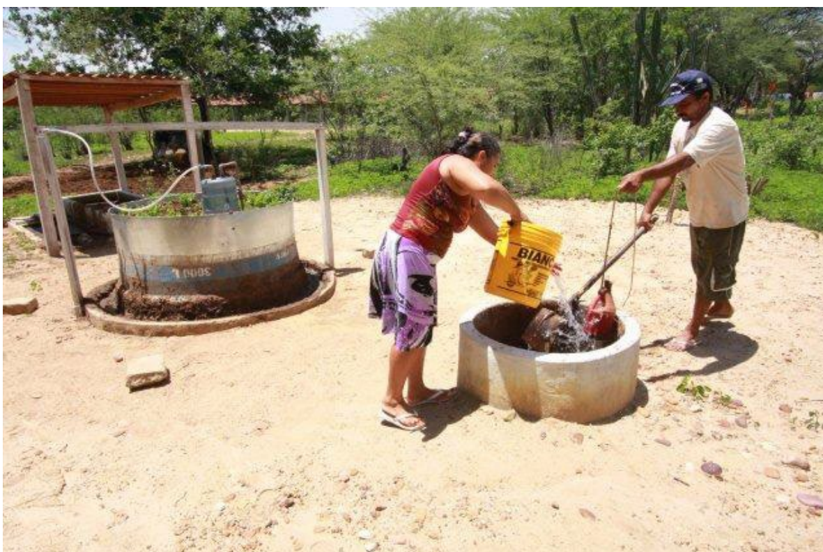
Photo D – Farmer couple, “loading” their biodigester with water and manure 307
