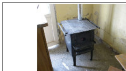
Figure 11 Improved wood stoves in Georgia (tested efficiency approx. 65%) (Ecovision, 2015)
