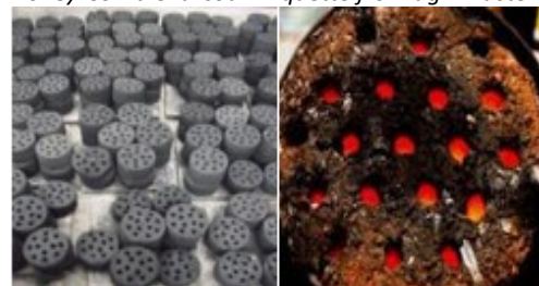
Honey-Comb Charcoal Briquette from agri-waste
