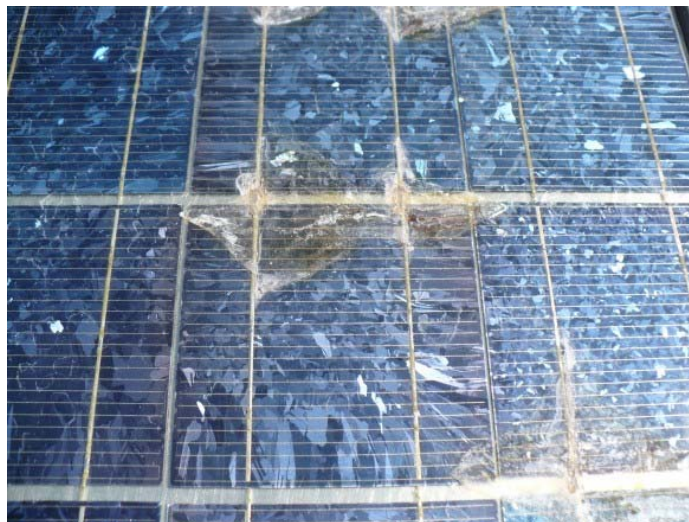
Figure 37: Panel failure due to cracking
