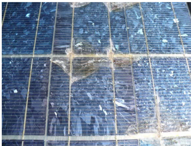
Figure 37: Panel failure due to cracking
