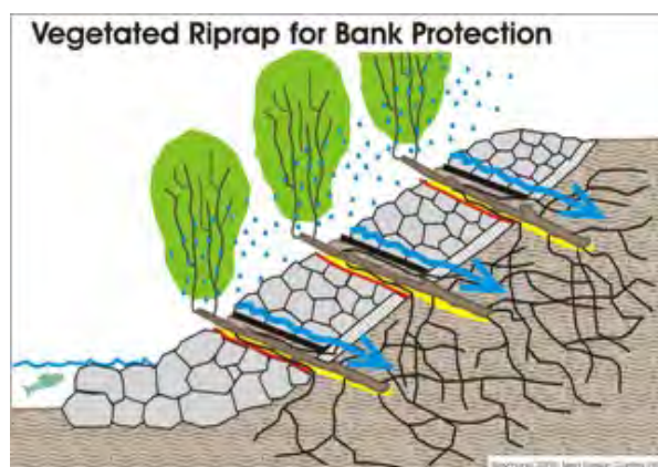
Figure 76: A model of vegetated riprap for bank protection
