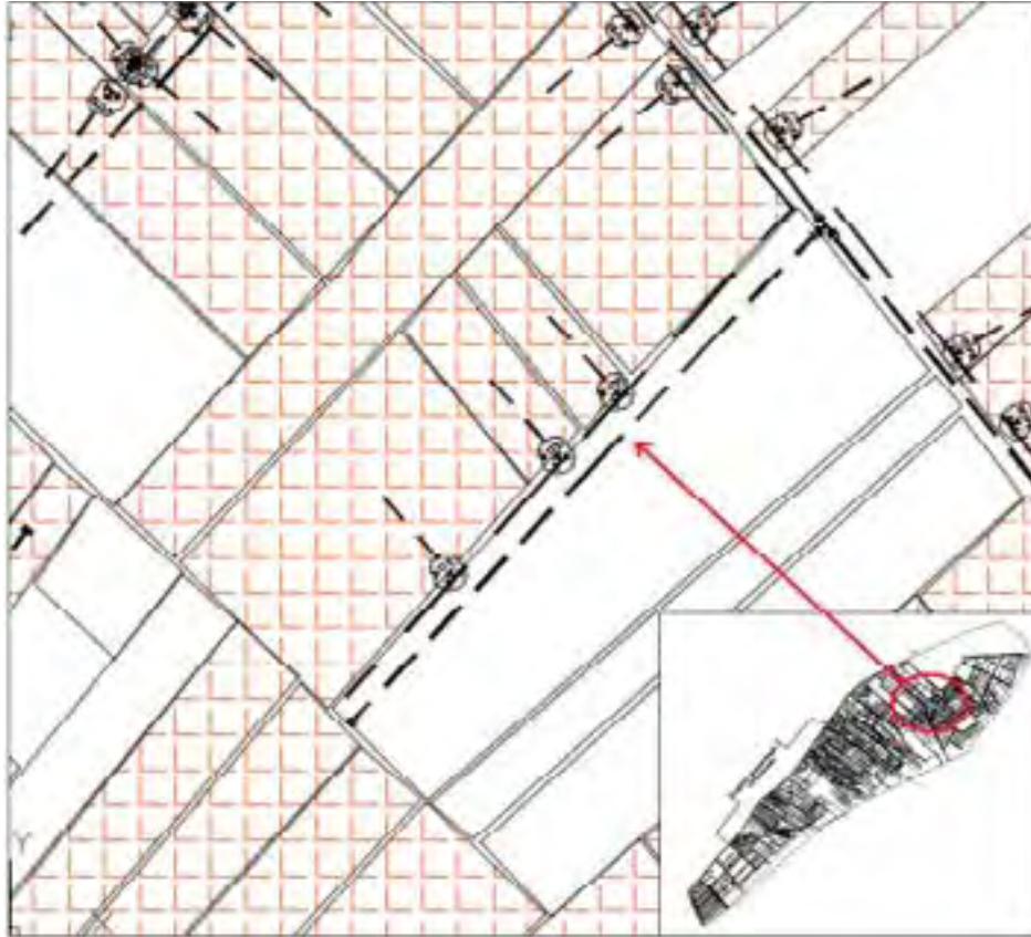
Figure 27: Arrow indicates two pipelines: ones with Farm connections and the other closed and apparently without a sense to exist
