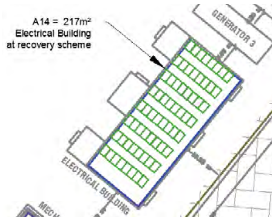
Figure 12-53: Variant 2 – example of a PV array on a roof-top area
