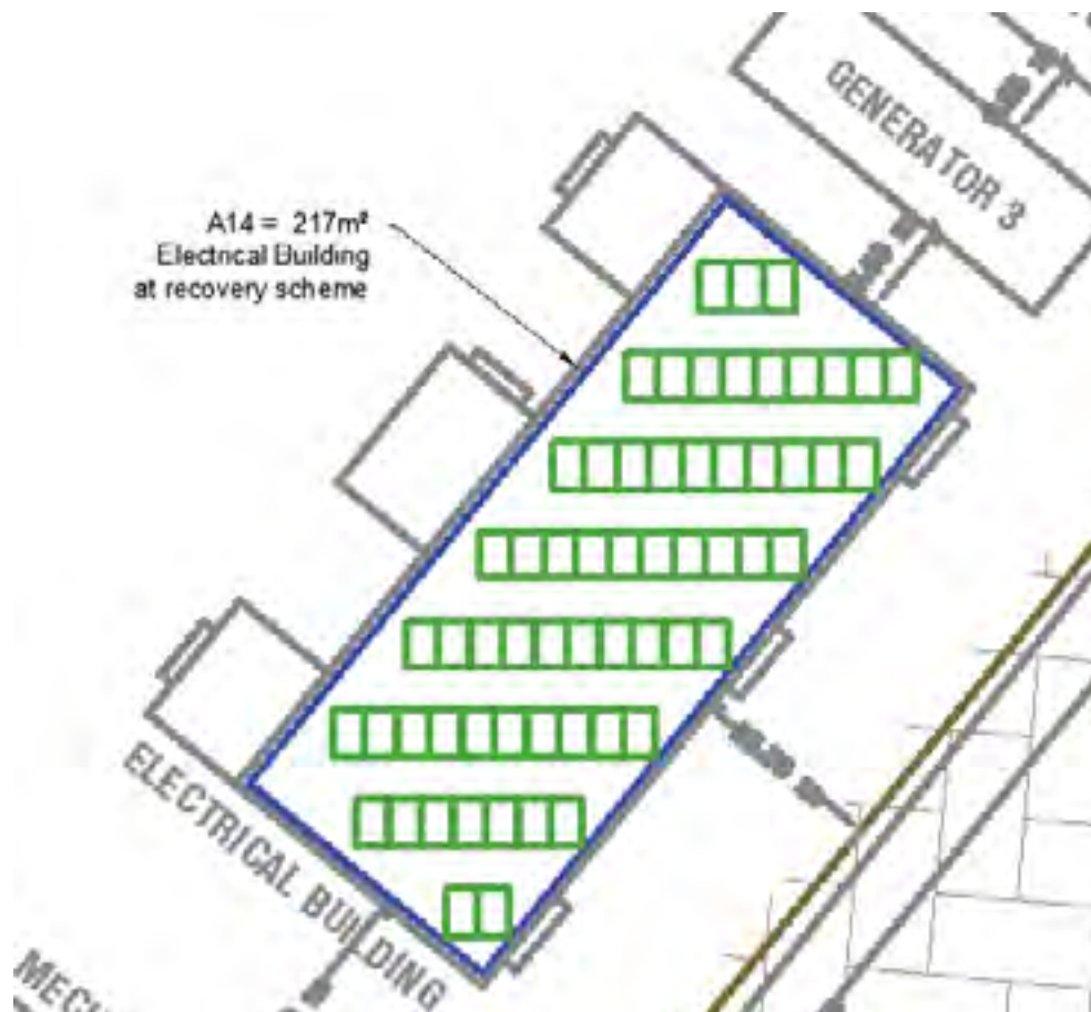
Figure 12-50: Variant 1 – example of a PV array on a roof-top area
