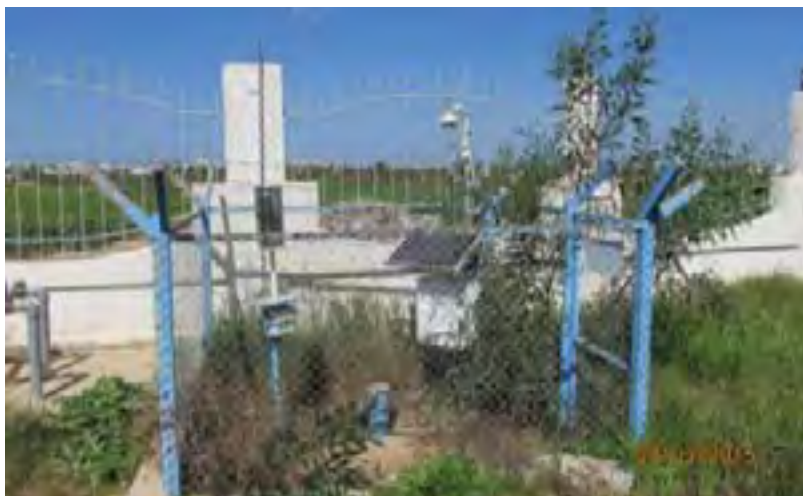
Figure 12-44: On-site meteorological station (no radiation measured)
