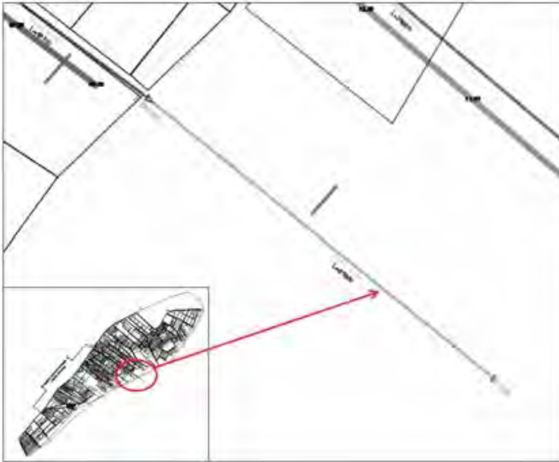
Figure 23 : Arrow indicates a pipeline very long extending about 200m further the last Farm Connection
